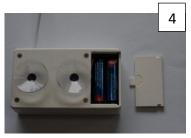
STEP 3 – Open the battery cover (4) and remove the insulator strip (5) to energize the unit. The unit will beep and the screen will display 'Hello' for 10 seconds and then 'Now waiting for Hot water' for a further 10 seconds. Replace the battery cover (6) and moisten the sucker pads on the rear of the control box. Fix the control box to the wall at an appropriate position by pressing up against the tiled surface (6)
