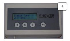
6. At the end of the shower, the Shower Shortener will provide some approximate statistics (Picture 5 and 6) including water used (based on time in the shower multiplied by the average flow of 9 litres/min). Approximate energy used to heat the hot water will also be briefly displayed. This approximate calculation is based on the approximate hot water used (assumes 60% hot water multiplied by a factor representing KWh/Litre to heat the water)
